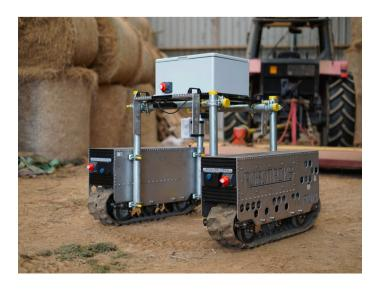
Built almost entirely out of aluminium with mounting surfaces on the top, front and rear of the traction units, the RTU was built to last when out in the elements. Featuring a low centre of mass and a wide footprint thanks to its tracked design, the RTU can drive in any orientation on surfaces up to a 54-degree incline.
